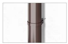
13. If it is necessary to mount the additional downspout fixing band directly on the downspout, allow for a movement of the downspout in the fixing band.
