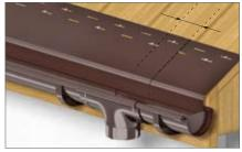
17. Eaves strips shall be hammered to the fascia board. Place the nails in the perforation provided. Allow for a 1mm-clearance between the strip and the nailhead. Strip shall be joint with a 8cm-overlap.
