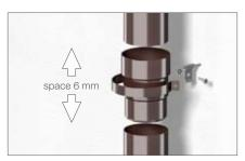
12. Use pipe connectors to join downspout sections. Downspout fixing bands shall be mounted to the neck of the connector. Allow for an about 6mm-space for the joints between the downspout sections and connectors.
