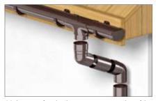
14. In case of projecting eaves a connection of the downspout and the drop outlet shall be done with the use of two elbows and a downspout section. If the connection of the drop outlet and an elbow is loose it should be fixed mechanically (with a screw or a rivet). Double-socket elbows may be used (and should be mounted with the arrow down).
