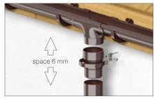
11. Install the downspout. Use a pipe connector to connect the downspout with the drop outlet. Downspout fixing band shall be mounted to the neck of the connector and fixed to the wall with a hook. The distance between downspout fixing bands shall be 2m.
