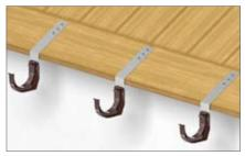
3b. It is possible to fix the brackets to the rafter or the eaves directly. To do this use steel rafter arms adapted to the roof pitch. The distance between neighbouring brackets shall not exceed 60 cm. Gutter fall is 0.3%..
