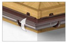
9. Install the corners. Insert the rear edge of the gutter into the rear fold of the corner. Then, turn the angle until its front edge snaps into the front edge fold of the fitting. The distance between the nearest hanger and the edge of the corner shall not exceed 15 cm.
