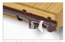
10a. Install left and right end caps. Insert the front edge fold of the end cap into the front gutter edge fold. Then, turn the cap upwards until its rear edge snaps onto the rear gutter edge fold. The caps should preferably be mounted on the gutter prior to the gutter is fixed to the hangers.
