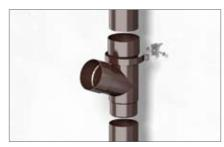
15. A pipe tee or a revision should be fixed to the wall with a fixing band and a hook. The fixing band shall be mounted at the connector. Allow for a 6-mm space.
