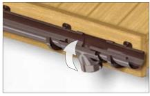
7. Install the drop outlet. Insert the rear edge of the outlet onto the rear gutter fold. Then, turn the outlet until its front edge snaps onto the front gutter edge fold. The outlet shall overlap the gutter fitting as per the designation on the fitting.
