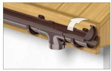
10b. A universal end cap can be used both for the left hand and right hand end of the gutter. Insert the front edge fold of the end cap onto the front gutter edge fold. Then, turn the cap down until its rear edge snaps into the rear gutter edge fold.
