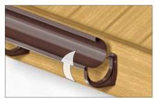
5. Install the gutters in the hangers. To do this insert the front edge fold of the gutter onto the front nibs of the hangers. Push the gutter towards the fascia board until its rear edge fold snaps on the rear hanger clip.
