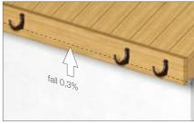
2. Fix the gutter hangers furthest from the drop outlet ensuring that the 0.3%-fall (3cm per 10m) is provided.
