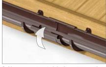
8. Use connectors to join the gutter sections (overlap as per the designation on the connector). The distance between the nearest hanger and the edge of the connector shall not exceed 15 cm.
