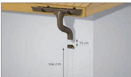
16. A downspout is fastened to the wall with a band and screws of different lengths. The maximum distance between fastening bands – 2 m. It is recommended to fasten each downspout to the wall using a minimum of two bands. Install the first band approx. 15 cm below the downspout elbow.
