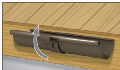
12b. Put the clamp on the front folds of elements connected, bend the protecting tab.
