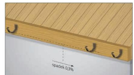
3. Install the gutter hangers furthest from the drop outlet ensuring that a minimum slope of 3 mm per 1 m is provided (recommended slope is 5 mm per 1 m).
