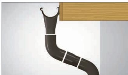
14. In the case of a protruding eaves, make the connection of a drop outlet with a downspout using two elbows and a downspout section.
