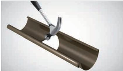
7. In the bottom part of the gutter, bend the hole edge down to provide better draining of water.
