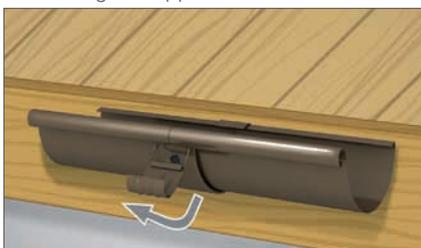
12a. The connection of gutters is sealed by installing gutter connectors on the gutter overlap. Engage the connector onto the rear edges of the elements connected, turn it up.
