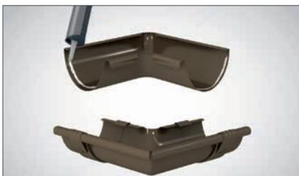
13. Similarly – as for the gutter connector – it is recommended to install a gutter corner. In this case, the gutters are inserted into the corner and the connections are sealed with gutter connectors. When mounting corners, it is recommended to additionally seal the overlap with a thin layer of universal roofing sealant.
