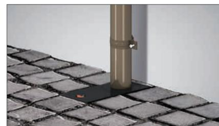
18. The downspout can also be introduced into a plastic catch basin, fitted with a strainer and anti-odour flap, to drain rainwater into a storm sewer.
