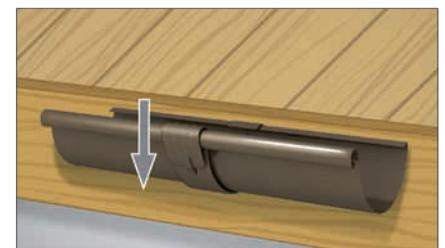
12c. Snap the latch and bend the protecting plate.
