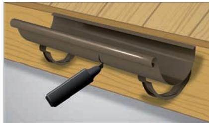
5. Place the gutter on the hangers and mark the location of a drop outlet.
